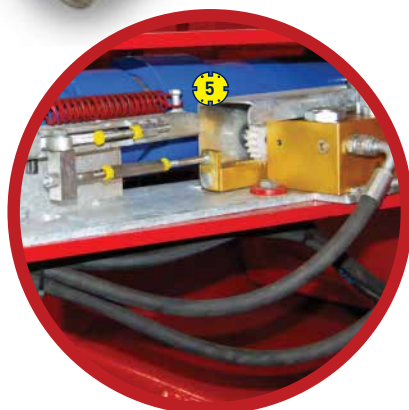
Front Main Ram & Speed Control Valve
