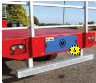
Recessed Lights, Rear Crash Barrier & Toolbox
