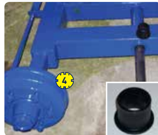
Oscillating Tandem c/w Devlon Bush
