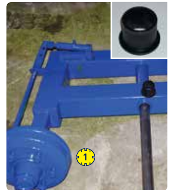
Optional Oscillating Tandem c/w Devlon Bush
